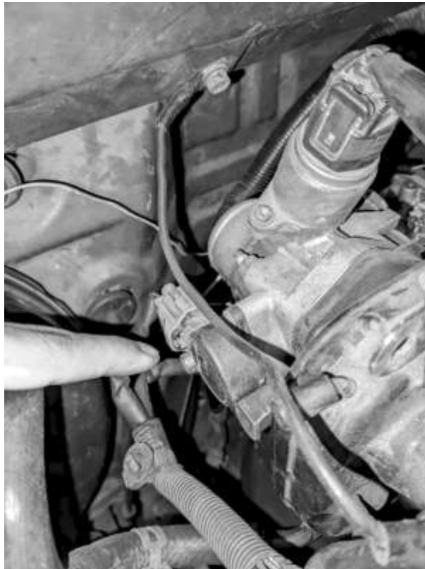
Figure 3. Throttle Position Sensor (TPS) documented during inspection
