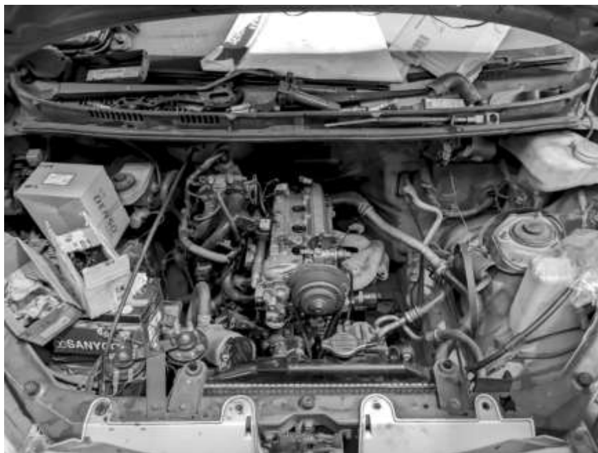
Figure 2. Daihatsu Xenia 1.0 Non-VVT-i engine used in the diagnostic case
