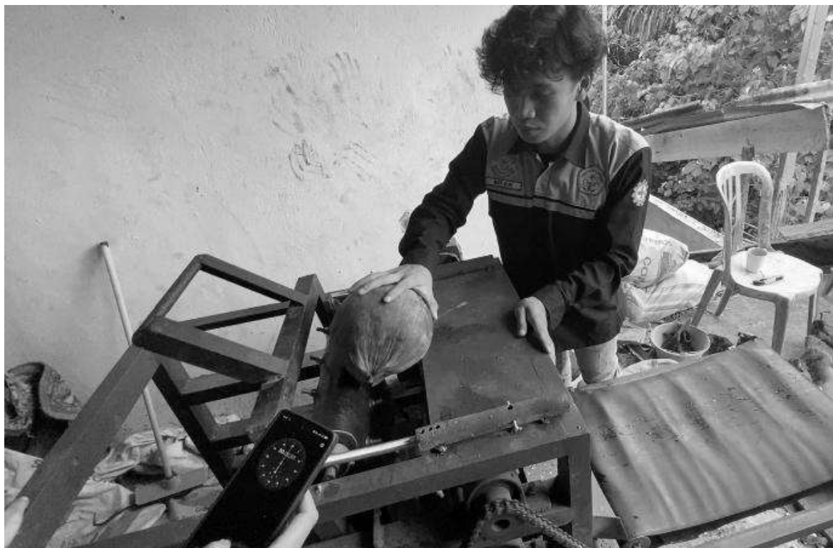
Figure 3. Functional testing of the developed coconut dehusking machine.
