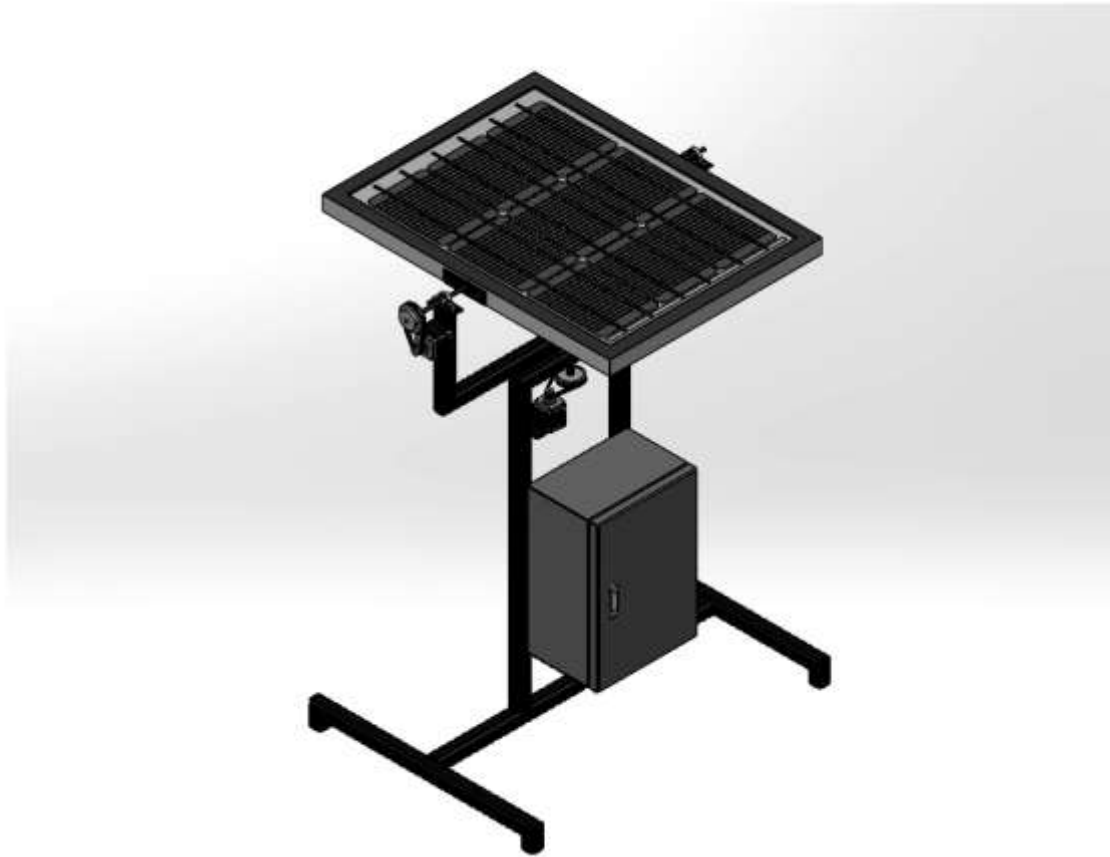
Figure 1. Conceptual Mechanical Design of the Proposed 50 Wp Dual-Axis Tracker
