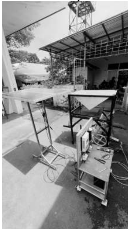
Figure 12. Assembled solar-powered paddy-husk separator prototype
