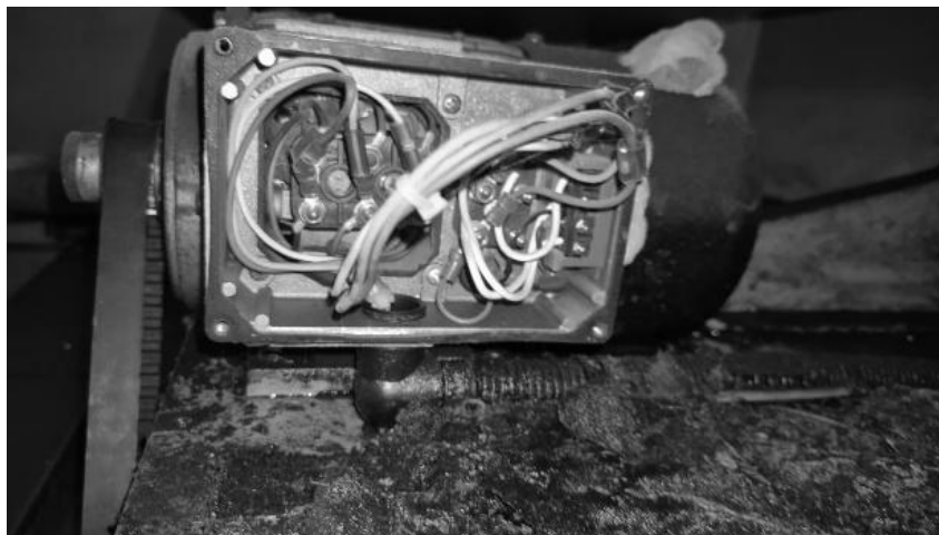
Figure 4. Motor stopper used as the workpiece guide limiter
