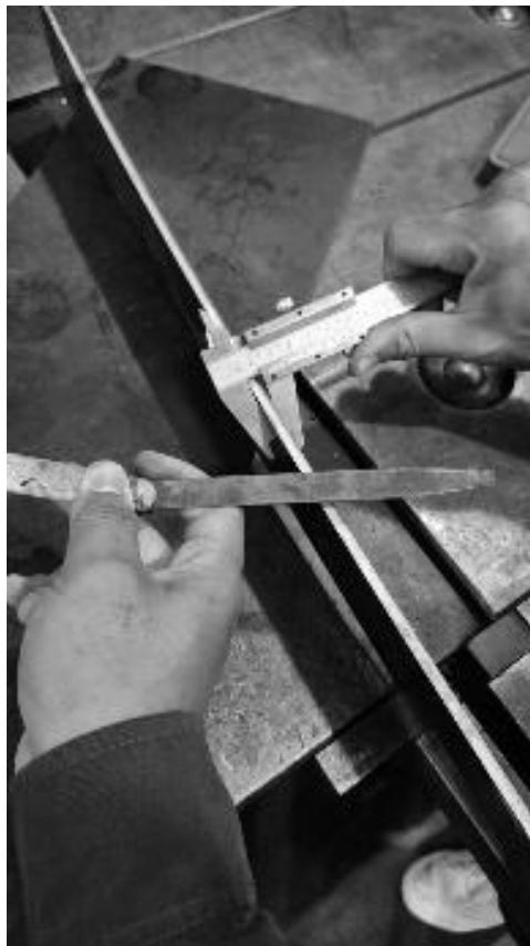
Figure 17. Post-retrofit cutting test on a 6 mm steel plate
