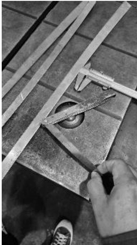
Figure 16. Post-retrofit cutting test on a 2 mm steel plate
