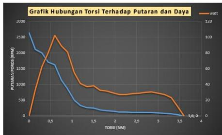
Figure 8. Condition  $Q = 0.06 \text{ m}^3/\text{s}$ , Head 50 cm, 4 blades, 40° angle, Standard Propeller Type.
