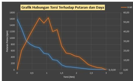
Figure 9. Condition  $Q = 0.06 \text{ m}^3/\text{s}$ , Head 50 cm, 4 blades, 40° angle, Plate/Straight Propeller Type.
